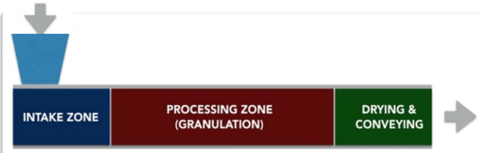
Fig. 3: Continuous Twin Screw Granulation Process
